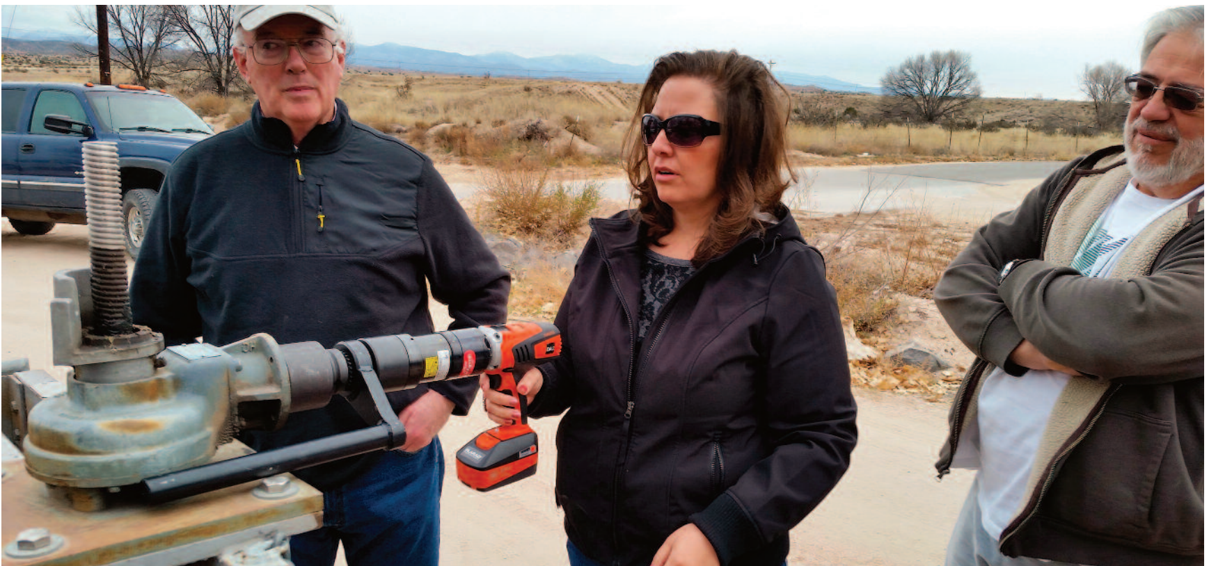
Acequia Madre de Alcalde Ingenuity: Lucia Sanchez, Commissioner of Acequia Madre de Alcalde, using the nut runner to open the headgate. Photo by Dick Williams.
